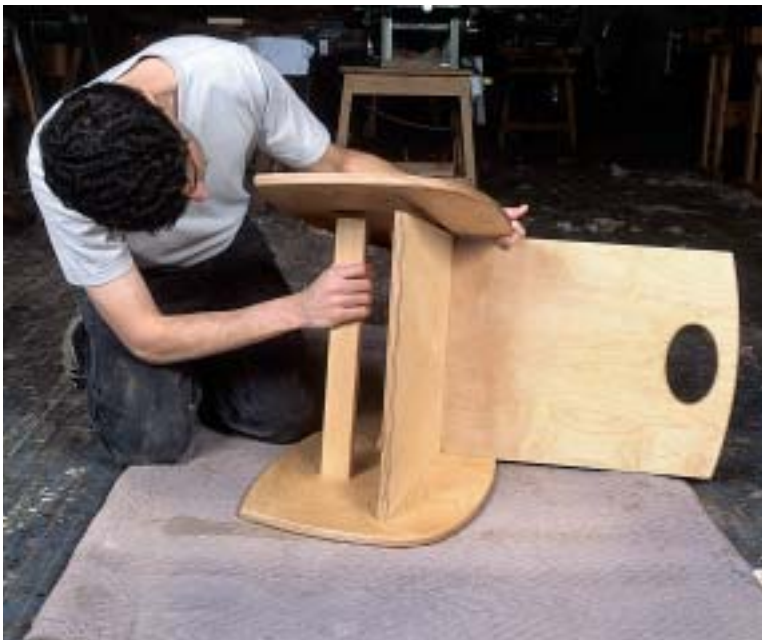
PHOTOS G AND H: Assembling the rocker can be frustrating without help. It makes sense to do it on a blanket or a piece of cardboard in case something slips apart.
