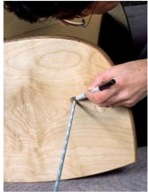
PHOTO I: Slip the threaded rod with one of the cap nuts all the way through the holes in one side and mark where the rod comes out the counterbore on the other side panel of the rocker.
