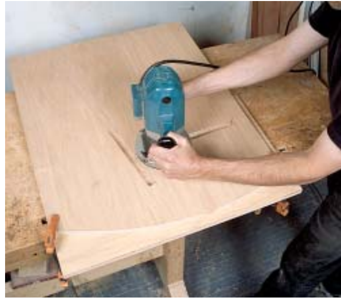
PHOTO B: The dados in the side panels are easy to rout, and they come out in exactly the right place if you use the dado jig.
