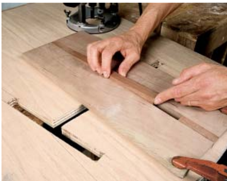
PHOTO A: A filler strip can be inserted in the interim dado jig to rout the short slot for the strut.
